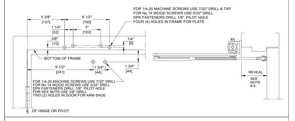
DOOR CLOSER MODELS: 7414, 7436 ARNPJ (NHO) TOP JAMB INSTALLATION (PUSH SIDE MOUNT) WITH PLATES BP74, BP86, BP86FC
